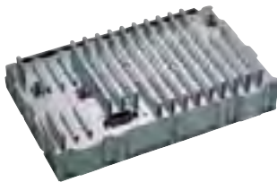
Power Amplifier Module of the Solid-State transceiver
